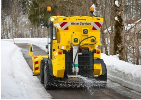
Figure 18 Multihog Winter Maintenance similar to that in use on Cambridge Guided Busway
